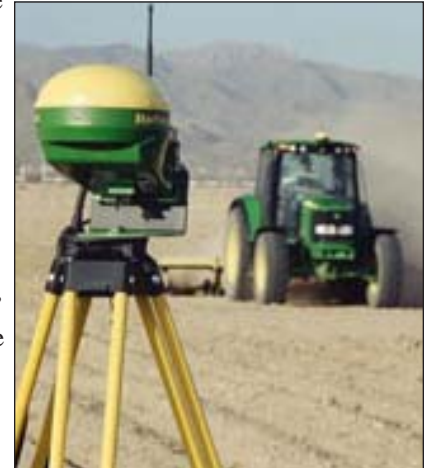
John Deere Ag Management Solutions (AMS) provides precision ag products such as GreenStar™ AutoTrac with RTK (Real Time Kinematic) that allows the operator sub-inch, repeatable accuracy when making passes through the field. Photo from JohnDeere.com
